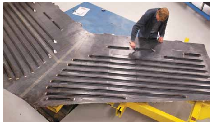
Fokker's 12m/39-ft span carbon fiber-PEKK torsion box demonstrator for TAPAS features integrated T-stiffeners.
